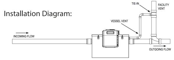
This guide provides an overview of optimal product installation practices. Refer to the manual for more installation options and detailed instructions. Equipment must be installed in compliance with all applicable laws, regulations and codes, including plumbing codes. Installation should be performed by a qualified plumber.
