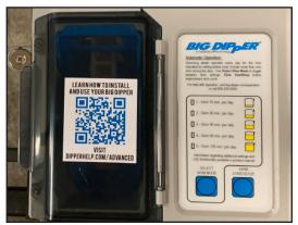
4. Close the new flip door. You should now be able to open and close the flip door to access the wiper blade for weekly maintenance.
