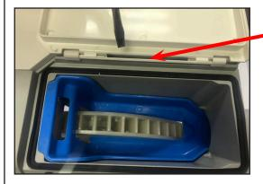
3. Place rubber gasket between metal pins. Use a flat head screwdriver to secure rubber if needed.
