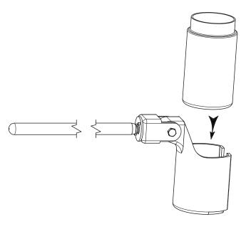
2. Adjust jar carrier to necessary angle for use with respective sampling port. Wing nut and bolt may be need to be tightened ocassionally to maintain position.
