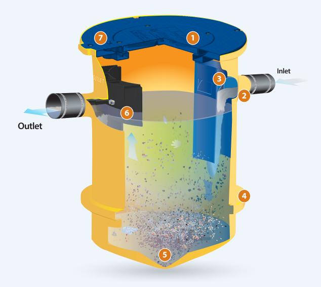
Solids-laden effluent from the kitchen flow is slowed and forced downward in a veritcal baffle, where solids filter out of the flow and sink to the bottom of the solids storage area. The "cleaned" effluent flows through the outlet. Pumping the Trapzilla® Solids Separator is easy—the pumper removes the lid and vacuums out the solids.
