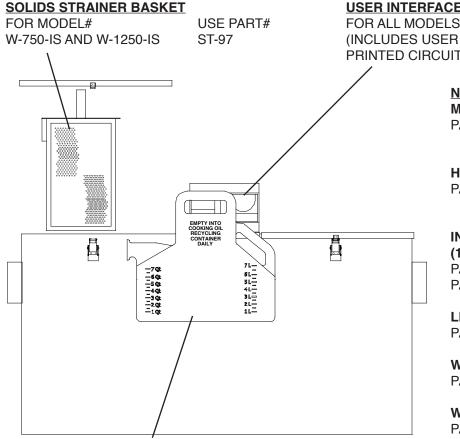
GREASE/OILS COLLECTION CONTAINER\* FOR MODEL W-750-IS, USE PART# GC-7 FOR MODEL W-1250-IS, USE PART# GC-6 (2)
